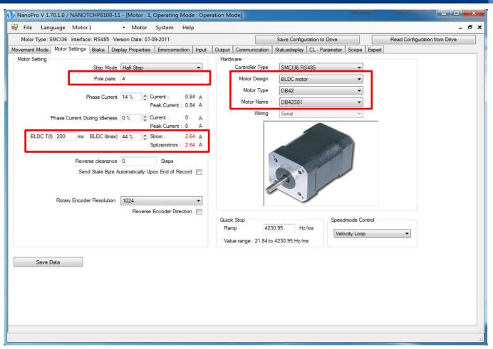
Special features for BLDC motors on the "Motor Settings" tab
