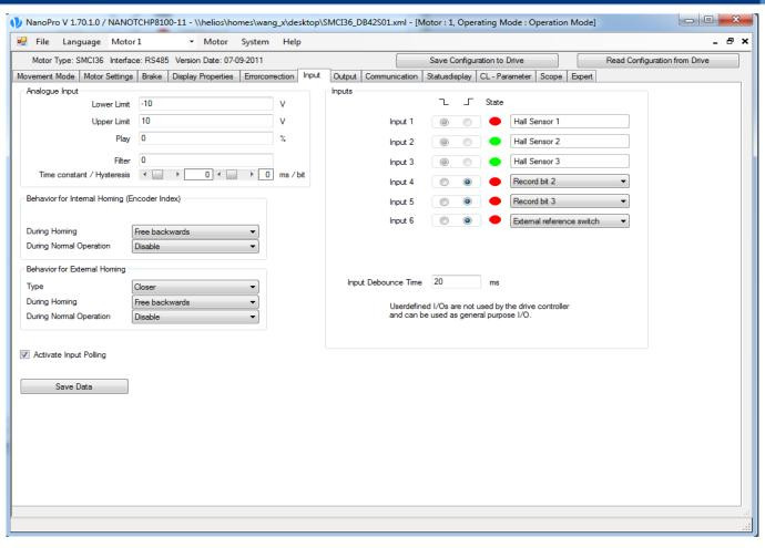
Special features for BLDC motors on the "Input" tab
