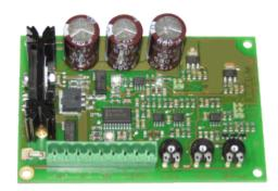
The controllers of series DR2.0 are suitable for closed-loop speed control operation of brush-type DC motors. 1-Q operation allows motor operation in one direction of rotation. EMF feedback with IxR compensation ensures speed consistency under load changes. The speed set point input accepts analogue voltages 0...10V, to be supplied through a potentiometer or by a plc analogue output. To supply an external potentiometer the DR2.0 provides a stabilized 10V voltage source.
